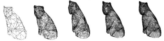
Fig. 7 Result of Applying Wavelet Transform : LOD = 0, 20, 40, 60, 100% (Cat)
